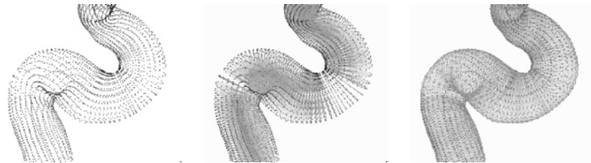
Figure 31. Topology of the vessel crawler showing: Masses (left), radial springs (middle), and stability springs (right) across sequential layers of the organism. See attached CD for color version.
